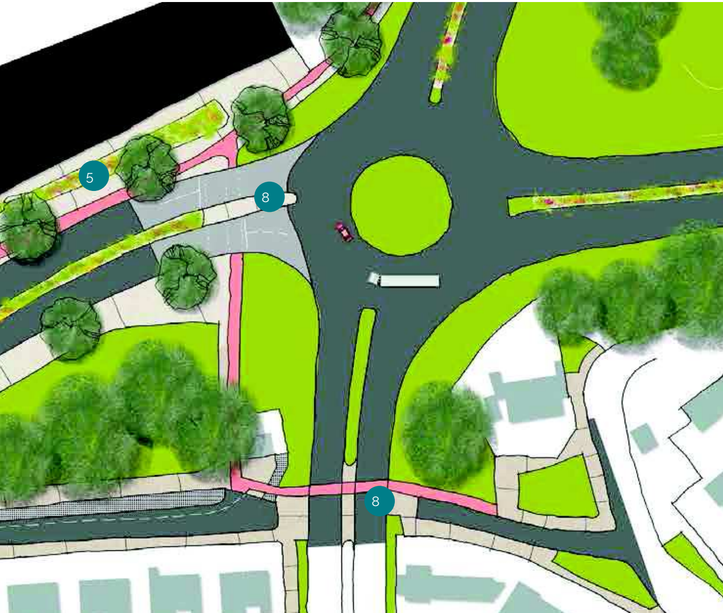
Figure 95. | illustration showing how an approach street environment might be designed to accommodate the mix of goals of allowing through traffic whilst prioritising good movement for pedestrians and cycling
