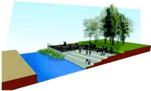
Figure 106. | river edges with retained wall edges, concrete construction slip access and steps
