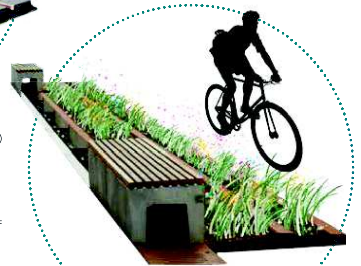
Figure 67. | examples of street sponge gardens that capture surface water and provide for planting of pollinators
